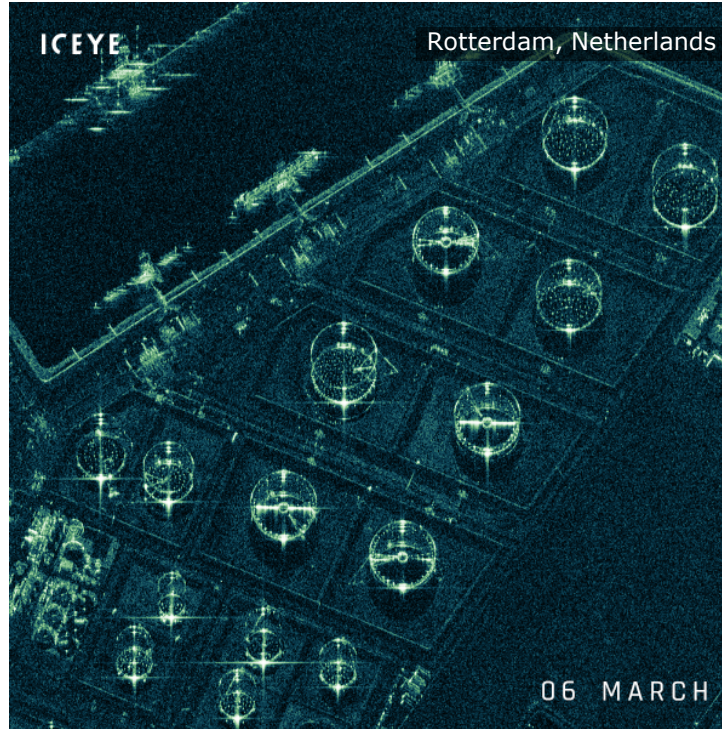
Time lapsed SAR images 2021 March 6–31 showing the movements of oil tank floating roofs and vessel traffic.
